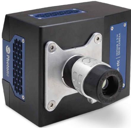
ZepHIR™ 2.9 is the only scientific-grade short-wave infrared HgCdTe (MCT) camera, ranging from 0.85 to 2.9  $\mu\text{m}$ . A four-stage TE deep-cooler, forced air-cooling at  $-80^{\circ}\text{C}$ , provides unrivaled low-noise levels at a 340 frame-per-second rate. Either it is for borehole samples analysis, pipeline gas detection, astronomy, space observation or material sorting, ZepHIR™ 2.9 extends the boundaries of laboratory and industrial imaging.
